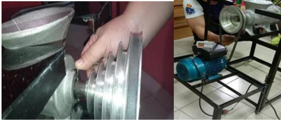
Figure 3. Pulley system for automatic shredding process
