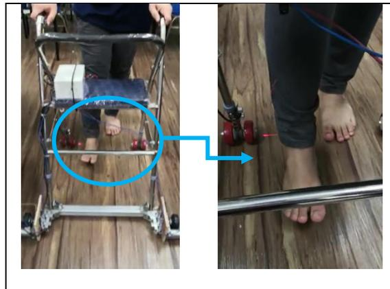
Figure 9. Subject stepping inside the laser guide
