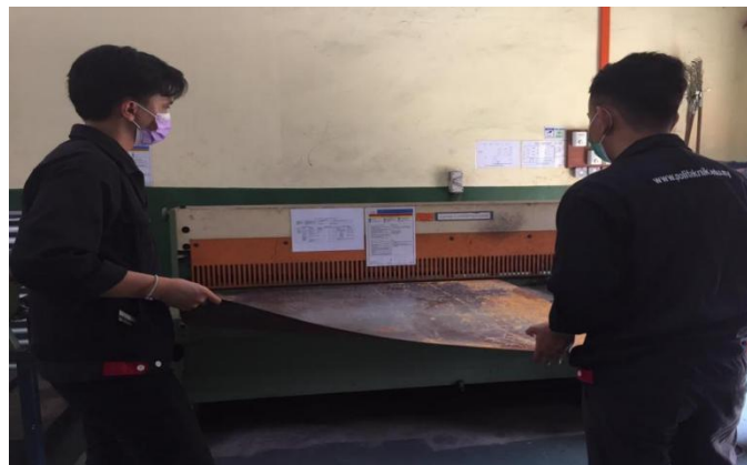
Figure 12. Cutting metal sheet
